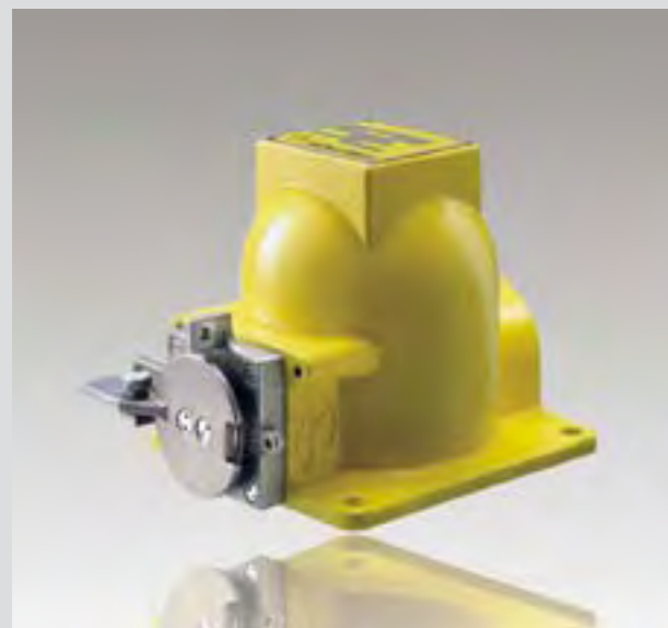
Under lock and key: The radioactive source sits in a multi-layered radiation protection container which protects the source capsule from damage. The radiation is focussed and directed in a narrow beam to the detector.
